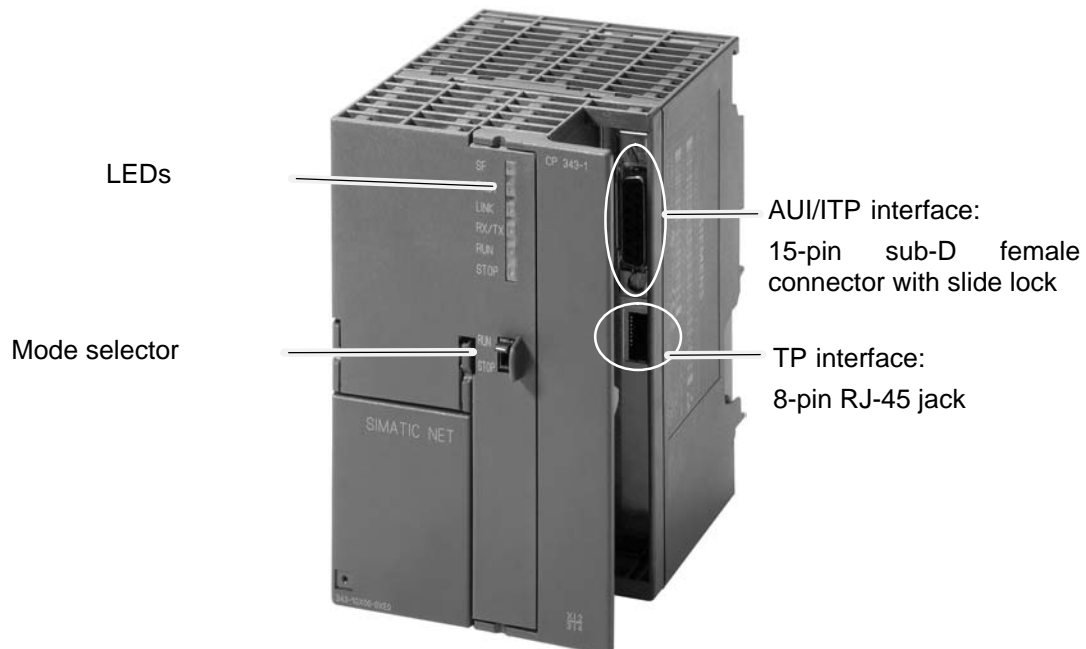
Figure 2-1 Front View of the CP 343-1
